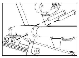
Figure 10: Attaching the handlebars
